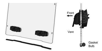
**2.** Push the gasket on the bottom of the windshield with the bulb section oriented as shown
