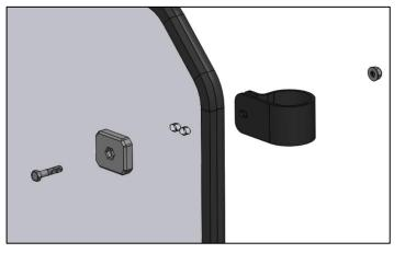
**3.** Snap 2 clamps on each side of the roll cage with the flanges facing forwards. Insert bolt through backing plates and windshield and loosely install nuts on all 4 clamps. Adjust windshield as needed and tighten nuts.
