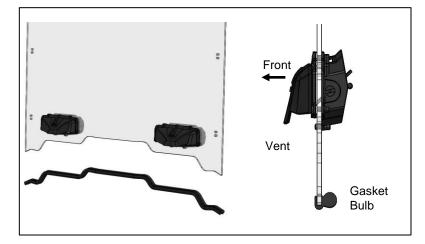
**2.** Push the gasket on the windshield starting at the center bottom with the bulb section oriented as shown. (Picture may not show exact windshield).
