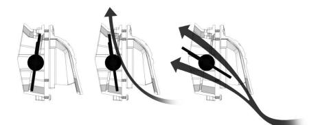
The vent has 3 positions: Closed, Defog, and open.
