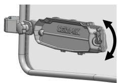
Turn handle to adjust vent. If the vent seems too tight or too loose, it can be adjusted by turning the T10 Torx screw in the handle.
