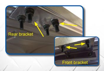
Connect the strut brackets to the top extrusion using 8mm carriage bolts, hand tighten hardware first. Once all bolts are in place then tighten.
