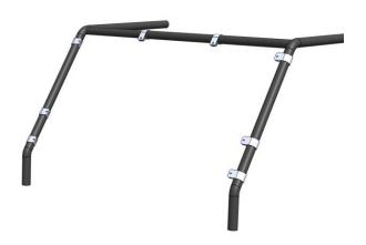
1. In the approximate locations shown, Snap 3 1.875" Plastic P Clamps on each side of the roll cage. The flanges will point forward and towards the center. Snap the smaller 1.75" clamps on the upper cross tube with the flanges forward and down.
