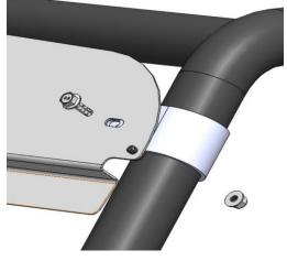
3. Bolt loosely in place using the M6x20 flange bolts and nyloc nuts.
